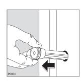
5. Place the machine in an upright position and remove the three plastic bolts.
